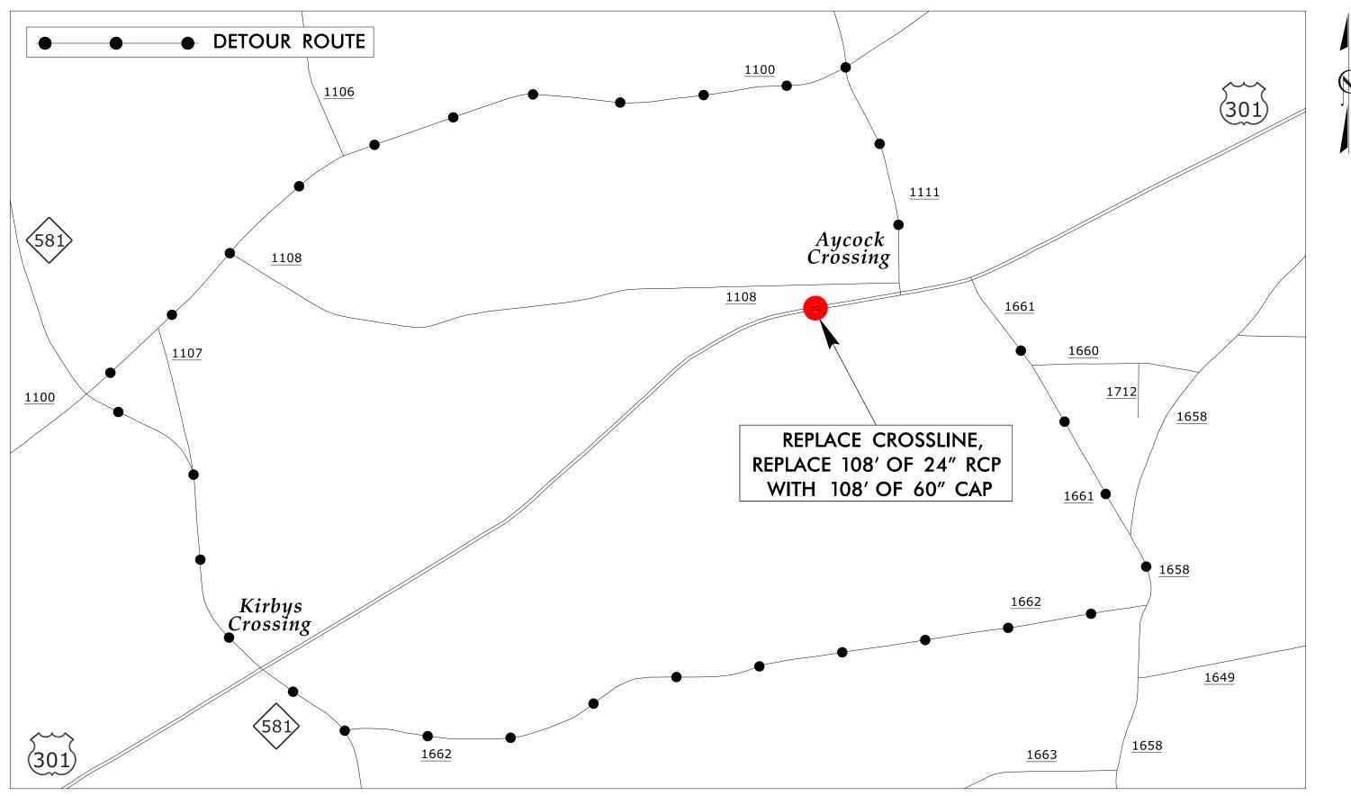
NOTE: SEE STANDARD DRAWINGS SECTION 1101.03 FOR TEMPORARY ROAD CLOSURES AND DETOURS
